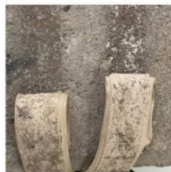
Figure 2 Substrate failure due to conditioning Score 3
